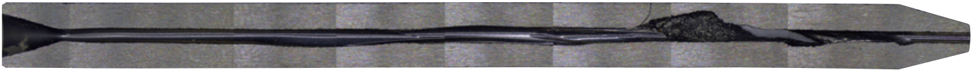
Completely worn channel as a result of severe misalignment. On the outside the nozzle is intact since the waterjet was stopped inside the nozzle.
